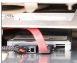
Internal 128 GB Solid State Disk for maximum reliability
